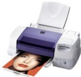
A monitor, a printer and a loudspeaker are all examples of output devices.
